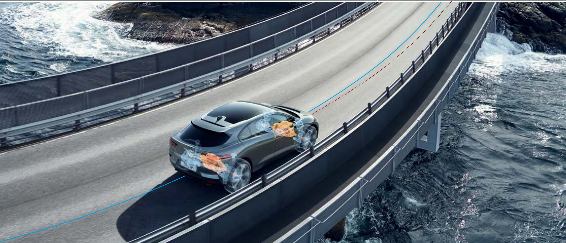
Torque Vectoring by Braking applies brake pressure to slow the inside front or inside rear wheels independently, helping to prevent understeer and stay on the true line of travel.
